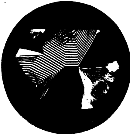
FIG. 136.—Section-plate of Amethyst Quartz, showing Sectorial Repeated Twinning of the Right and Left Varieties
